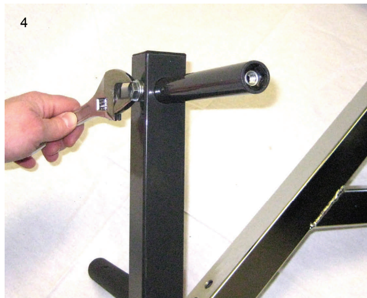
Step 4: Insert the ROLLER PAD TUBE and secure with the M10 bolt and M10 washer.
