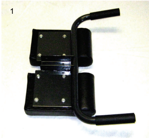
Step 1: Assemble THIGH PADS to the HANDLE FRAME using the eight 5/16" bolts and eight washers. Do not over tighten.
