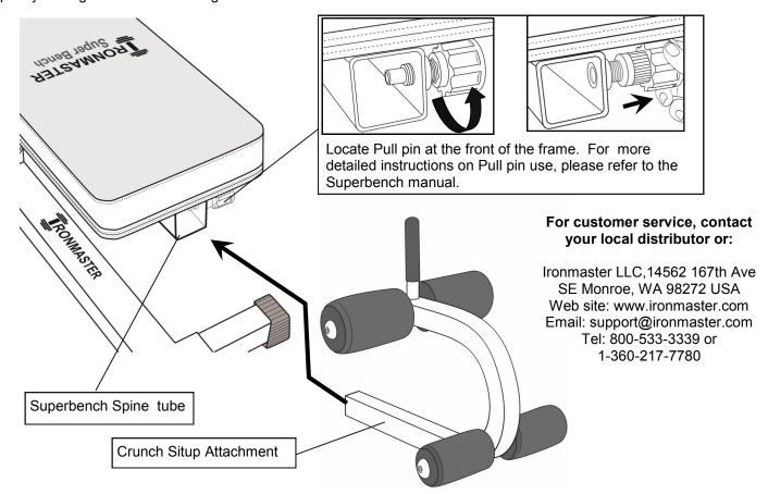
**WARNING:** Never under any circumstances use any of the Super Bench accessories with either a faulty or missing pull pin in conjunction with the Super Bench. Serious injury could occur. If the Pull pin fails to operate correctly or for any reason, fails to locate properly with the Ironmaster Crunch Situp accessory, discontinue use and contact your nearest dealer. This attachment is only for situp/crunch exercises or decline bench presses. Do not use for other purposes.
