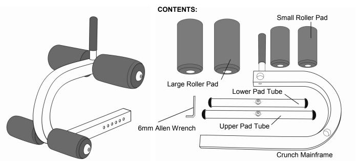
ASSEMBLY: Check that all parts are present. Note that Allen Bolts, Round Caps, Flat washers and 4x Black Allen Head bolts are pre-installed on the Upper/Lower pad tubes. With the supplied 6mm Allen Wrench, remove the M12 Allen Head bolts from the middle of the Upper/Lower Pad tubes and all four of the Round Cap/ Black Allen Head assemblies Slide Upper/Lower Pad Tubes into their prospective positions on the Crunch Main frame as shown blow and tighten bolts.
