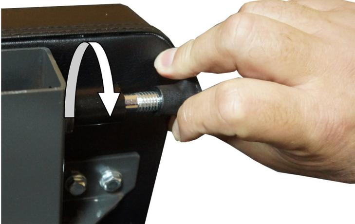
Locate the PULL PIN which is under the front of the seat pad. Unscrew the PULL PIN until the Pin is in the unlocked position. Pull the PULL PIN and slide the CABLE TOWER SEAT onto the Cable Tower stub.
