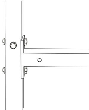
Once the PULL PIN snaps into the stub hole, tighten the PULL PIN to the locked position and make any necessary adjustments to seat height or leveling using the methods show on previous page.
