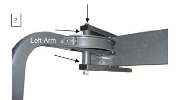
Insert Bearing Flanges on the top and bottom of each Arm and push the Arm into position inside the Bearing Housing frame. Attach with M10 long bolts, washers and lock nuts. Do not over tighten—the Arms should pivot freely.
