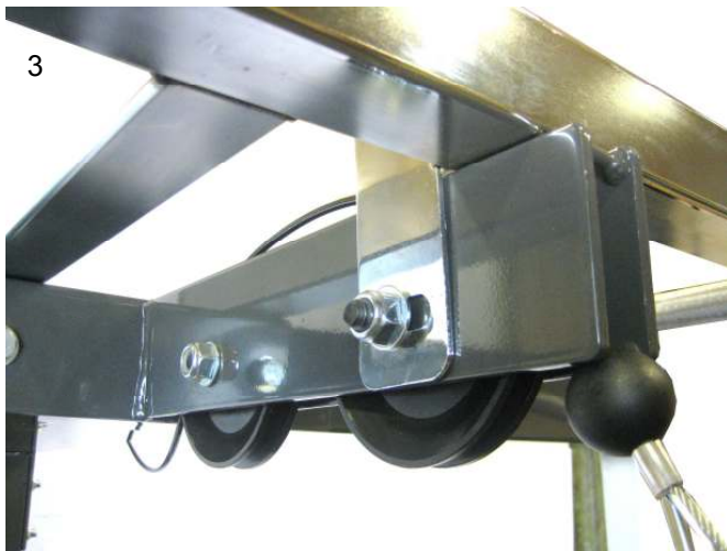
Step 3: Insert M12 x 60 Allen bolt through Crossbar front tabs and reinstall the pulley wheel. Use washers on both sides and hand tighten nut. Then fully tighten all three bolts and nuts using two wrenches so the lock nuts are seated tightly.
