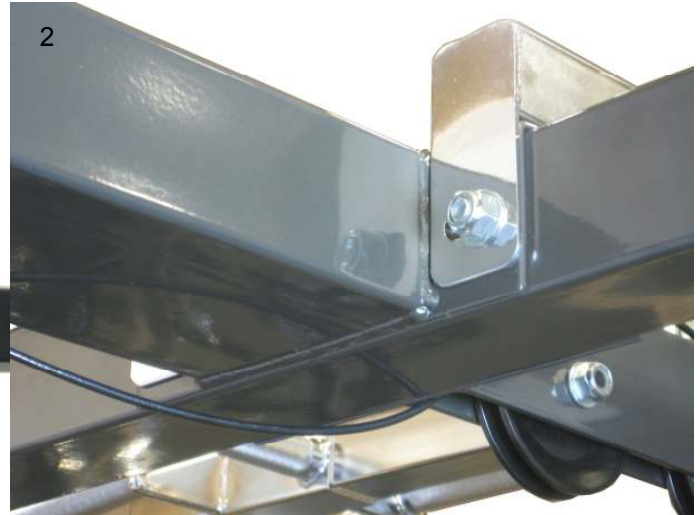
Step 2: Set Crossbar frame over the top of the IM2000 machine and insert the M12 x 100 bolts through the top center bracket and crossbar rear tabs. Use washers on both sides and hand tighten the nuts.
