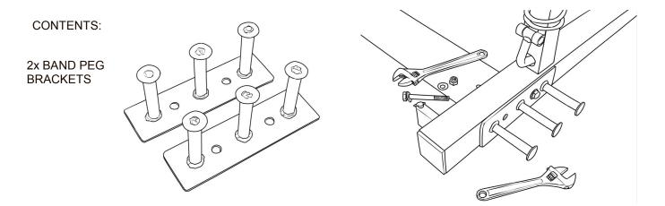
**Assembly:** Remove existing M12 bolts from the frame of IM2000 BASE as shown. Align BAND PEG brackets over existing bolt holes with BAND PEGS facing outward.
